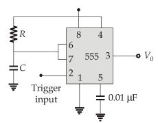
The output of the monostable multivibrator using 555 timer remains in its stable state until it gets a trigger. We have,
