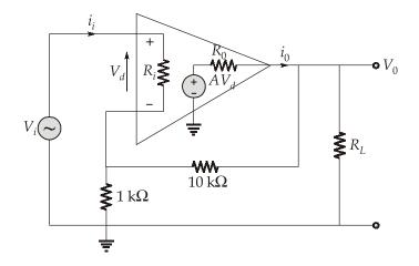
$$V_d = V_i - V_0 \left(\frac{1}{10 + 1}\right) \tag{1}$$
