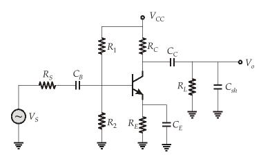
where,  $C_E$  = Emitter bypass capacitor
