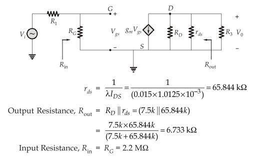
The small-signal equivalent representation for the amplifier is as shown below:
