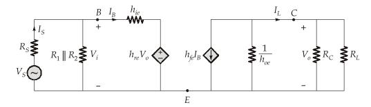
$$V_0 = -(h_{fe}I_B) \times R_L''$$
