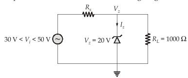
For zener diode to be in breakdown region,  $V_z > 20 \text{ V}$ .
