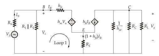
$$V_0 = -(h_{fe}I_B) \times R_L''$$
