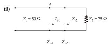
For  $\frac{\lambda}{4}$  transformer the input impedance is given by,  $Z_{in} = \frac{Z_o^2}{Z_I}$
