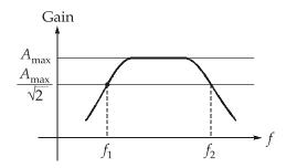
In the bandpass filter, the low pass section defines the upper cut-off frequency  $f_2$  = 4 kHz and high pass section defines the cut-off frequency  $f_1$  = 2 kHz.
