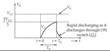
Suppose at t = 0, the trigger input is applied and the capacitor starts charging through resistance R. When capacitor is charging,
