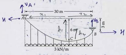
minimum tension at C [12 marks] max'm tendion at A
