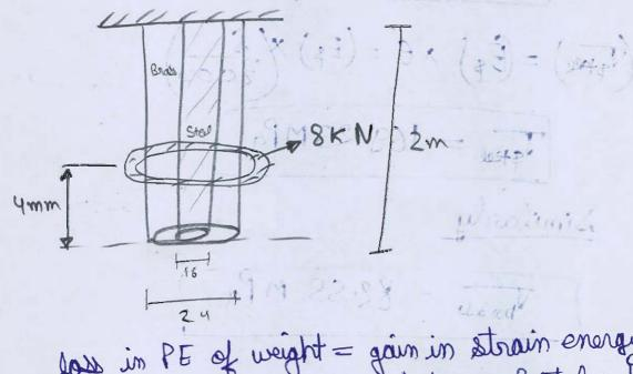
loss in PE of weight = gain in strain energy of brass & steel nod
