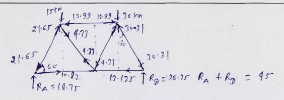
$R_0 \times 6 = 15 \times 3 + 30 \times 4.5$   $R_0 = 18.75 \text{ EN}$
