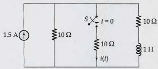
If switch *S* is closed at t = 0, calculate i(t) for t > 0 by using Laplace transform approach. [10 marks]
