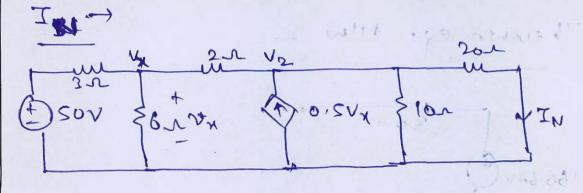
$$\frac{50 - v_{x}}{3} = \frac{v_{x}}{6} + \frac{v_{x} - v_{z}}{2}$$
