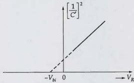
Assume that the intercept of the curve on the voltage axis in above figure gives -0.855 V and that the slope is  $1.32 \times 10^{15}$  (F/cm<sup>2</sup>)<sup>-2</sup>V<sup>-1</sup>.
