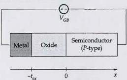
The oxide thickness,  $t_{ox} = 50$  nm and the doping level in the p-type substrate is  $N_a = 10^{16}$  cm<sup>-3</sup>. Assume, intrinsic carrier concentration of semiconductor,  $n_i = 10^{10}/\text{cm}^3$ , thermal voltage,  $V_T = 26$  mV,  $\epsilon_{\text{oxide}} = 3.45 \times 10^{-13}$  F/cm,  $\epsilon_{si} = 1.05 \times 10^{-12}$  F/cm. Calculate the hole concentration, p at the oxide-semiconductor interface (i.e., x = 0) under the following conditions:
