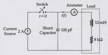
Initially, when the switch is open, the capacitor is discharged and the ammeter reads zero ampere. After the switch is closed, the ammeter reading keep fluctuating for some time till it settle to a final steady value. Calculate the maximum ammeter reading that one will observe after the switch is closed.
