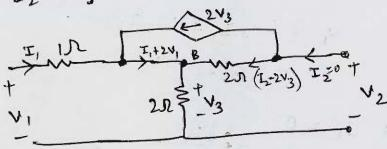
Applying KVL at input side
