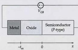
The oxide thickness,  $t_{ox} = 50$  nm and the doping level in the p-type substrate is  $N_a = 10^{16}$  cm<sup>-3</sup>. Assume, intrinsic carrier concentration of semiconductor,  $n_i = 10^{10}/\text{cm}^3$ , thermal voltage,  $V_T = 26$  mV,  $\epsilon_{oxide} = 3.45 \times 10^{-13}$  F/cm,  $\epsilon_{si} = 1.05 \times 10^{-12}$  F/cm. Calculate the hole concentration, p at the oxide-semiconductor interface (i.e., x = 0) under the following conditions:
