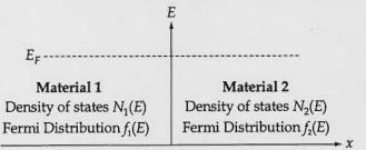
Assume the net motion of electrons is zero, show that the equilibrium Fermi level must be constant throughout, that is,  $E_{F_1} = E_{F_2}$  (or) show that no gradient exists in the Fermi level at equilibrium,  $\frac{dE_F}{dx} = 0$
