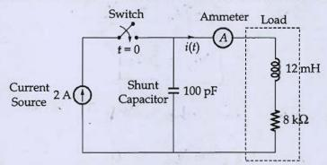
Initially, when the switch is open, the capacitor is discharged and the ammeter reads zero ampere. After the switch is closed, the ammeter reading keep fluctuating for some time till it settle to a final steady value. Calculate the maximum ammeter reading that one will observe after the switch is closed.
