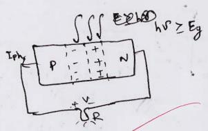
when light falls on the depletion region of the P-n junction, then large amount of the pariers (electron hole pairs) are generated (Energy of inerdent photon should be greater than bandgap (Eg) of the semiconductor.
