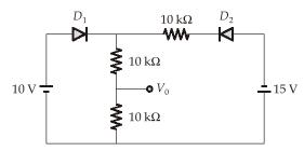
We can observe that diode  $D_2$  is always off so equivalent circuit is
