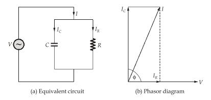
• The material to be heated may be considered imperfect dielectric of a condenser and may be, therefore represented as a capacitance placed in parallel with a resistance as shown in Fig. (a). The phasor diagram of the circuit is shown in Fig. (b). If V is the supply voltage, f is the supply frequency in Hz, cosf is the power factor of the load and C is the capacitance of the condenser in Farads.
