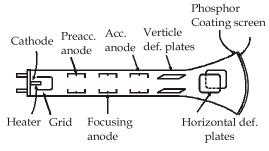
• CRT works on the principle of thermionic emission i.e. emission of electrons from a heated surface. The various part of CRT are discussed below:
