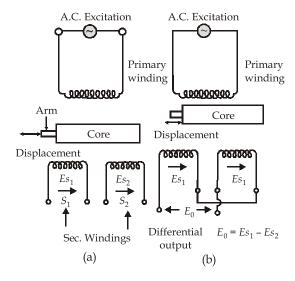
• LVDT is the most widely used inductive transducer for converting the linear into proportional output electrical voltage.
