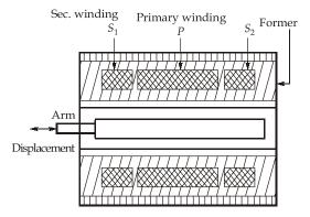
Linear variable differential transformer (LVDT):
