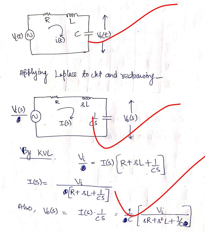
$$V_{\delta}(s) = \frac{V_{i}(s)}{e^{2}LC + sRC + 1}$$
