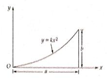
$\rightarrow$  Let us consider a strip of dr | 12 marks| dx b thickness at a distance x from enigin  $f(x) = kx^2$   $\rightarrow$  centroid of the small strip is at - Let us consider a strip of de ✓ a distance of x grom origin.
