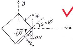
Assuming x', and y' as original regrence plane axes- $\sigma_{n} = \frac{\sigma_{x'} + \sigma_{y'}}{2} \cos 20 + \frac{\sigma_{x'} - \sigma_{y'}}{2} \cos 20 + C_{x'y'} \sin 20$
