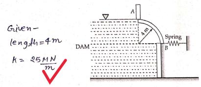
[20 marks] FH Fr 28 Projecting the covered sibme Porojecting the conved sibmerged surface on a vertical plane
