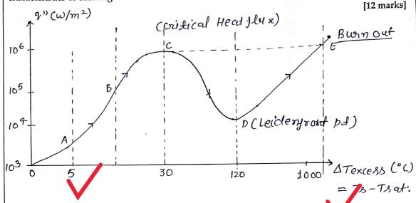
→above figure shows pool Boiling or Natural Boiling of stationary fluids such as water. → x-9xis represents temp. difference between surface and saturation temp at a particular priessure, and 4 aris represents heat plux through the swyace to stationary fluid. OAB Region - 6A)gt is Natural convection Boiling region. 59n this region bubbles forming due to vaporization of water quickly collapse and do not rise upto free surjage of water. Region - In this region Wadeate Boiling takes
