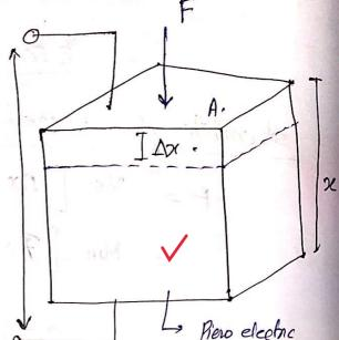
one those on which if the normal applied & then they get deformed and corresponding to it the output voltage
