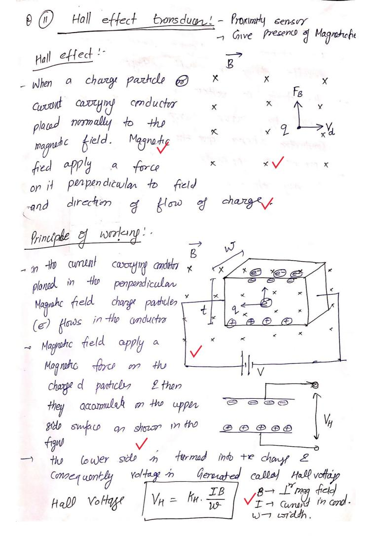
Magnetic field occurs, it As change in results change in hall voltage the change in voltage is \* sensed by current carryy Conductor Ehence give the presence @ Absence object. make full figure with naming if you are making
