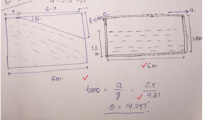
Applying man conservation intial empty Tank volume = final empty tank vol"  $0.6 \times 6 = \frac{1}{2} \times (6 - \pi) (6 - \pi) \tan (4.297)$  $7.2 = (6-\pi)^2 \tan 14.297$  $\chi = 0.6046 m$ Calculation of Total Pressno force x. A @ upper vall Let PA = Sa.x + Patm. Pahm effect is not taken since it is working on both side.  $P_{A} = Sa\chi.$   $\int dF = \int P_{A} dx. w$ = 1000 × 2.5×1 xd7.  $F = 1000 \times 2.5 \left[\frac{\pi^2}{2}\right]^{0.6846}$ F = 585.84N Am X
