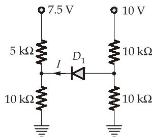
If the cut-in voltage of the diode  $D_1$  is equal to 0.7 V, then the value of current flowing through the diode is
