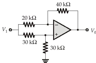
The value of output voltage  $V_0$  is equal to
