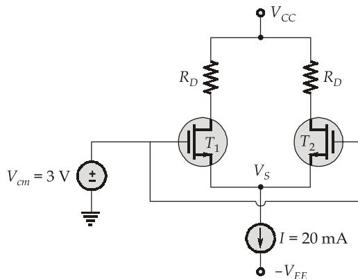
The two transistors are exactly matched with  $V_t = 0.5$  V,  $\mu_n C_{ox} = 500 \mu\text{A}/\text{V}^2$  and  $\left(\frac{W}{L}\right) = 100$ .
