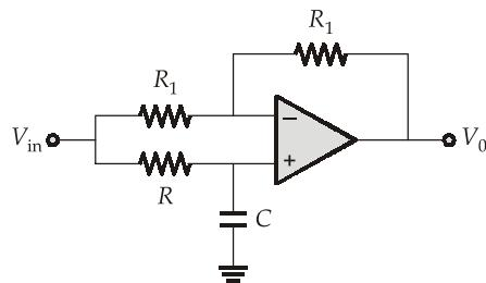
the maximum phase shift possible in output of the circuit is
