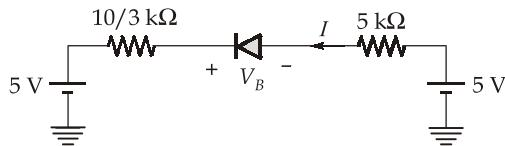
Applying KVL we get  $V_D = 0$  V, thus no current will flow through the diode  $D_1$ .
