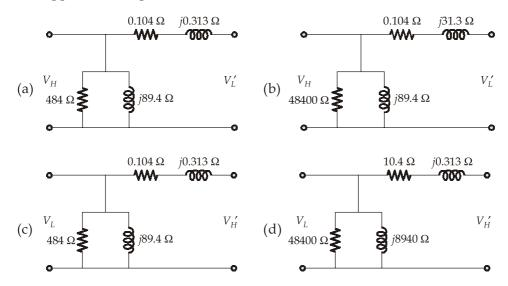
Q.118 A 1-φ, 3 kVA, 240/120 V, 60 Hz transformer has the following parameters:
