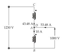
kVA rating = series winding current × voltage
