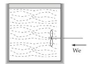
$$\begin{aligned} W_e &= 440000 \\ \delta Q &= \Delta U + \delta W \\ mc_v(T_2 - T_1) &= W_e \\ 1 \times 800 \times (T_2 - 50) &= W_e \\ 800 \times (T_2 - 50) &= 440000 \\ T_2 &= 600 \text{ K} \end{aligned}$$
