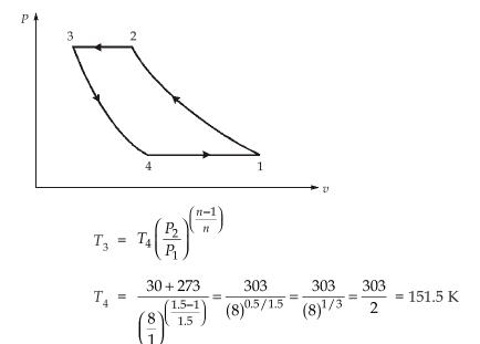
Heat extracted from the cold chamber =  $c_n(T_1 - T_4) = 1(283 - 151.5) = 131.5 \text{ kJ/kg}$
