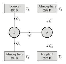
$Q_3$  is the heat removed by the refrigerator to produce the required ice.
