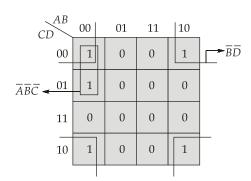
$$f = \overline{A}\overline{B}\overline{C} + \overline{B}\overline{D} = \overline{B}(\overline{A}\overline{C} + \overline{D})$$
