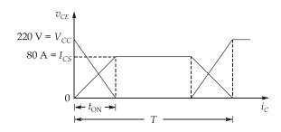
$$P_{\text{loss}} = \frac{V_{\text{CC}}I_{\text{CS}} \times t_{\text{on}}}{6} \times f$$
