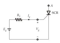
Gate power dissipation,  $P_g = V_g I_g = 0.65 \text{ W}$
