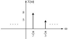
The frequency components in the spectrum are integer multiples of the fundamental frequency  $\omega_0$ . Thus, the fundamental frequency,
