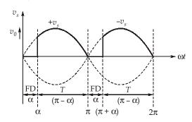
The FD conducts two times in 1 cycle
