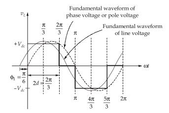
i.e. the fundamental line voltage leads the fundamental pole voltage or phase voltage by  $\frac{\pi}{6}$  radians
