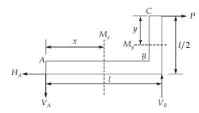
$$= \int_{0}^{l} \frac{M_{x}^{2} dx}{2EI} + \int_{0}^{l/2} \frac{M_{y}^{2} dy}{2EI} = \int_{0}^{l} \frac{\left(-\frac{Px}{2}\right)^{2} dx}{2EI} + \int_{0}^{l/2} \frac{\left(Py\right)^{2} dy}{2EI}$$
