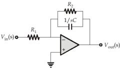
$$\frac{V_0(s)}{V_i(s)} = \frac{-R_2 \parallel \left(\frac{1}{sC}\right)}{R_1}$$
