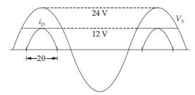
The diode conducts when  $V_s$  exceeds 12 V, as shown above, The conduction angle is 2  $\theta$ , where  $\theta$  is given by
