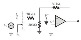
$$R_i = \frac{V_s}{I_l} = 20 \text{ k}\Omega$$
