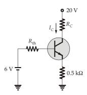
The operating state of BJT will be decided by value of  $R_C$ . According the value of  $R_C$ . BJT may be in active state or saturation state. So,  $I_{\rm C}$  can not be found out.
