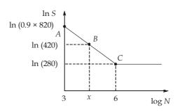
Since ABC is a straight line, so slope of AC = slope of BC
