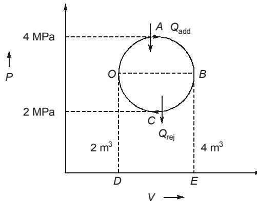
In cycle  $Q_{\text{net}} = W_{\text{net}} = \text{Area enclosed by cycle.}$
