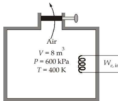
$$m_1 = \frac{P_1 V_1}{R T_1} = \frac{600 \times 8}{0.287 \times 400} = 41.81 \text{ kg}$$
