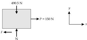
Because  $P \le F_{\text{max'}}$  we conclude that the block is in static equilibrium and correct value of friction force is,
