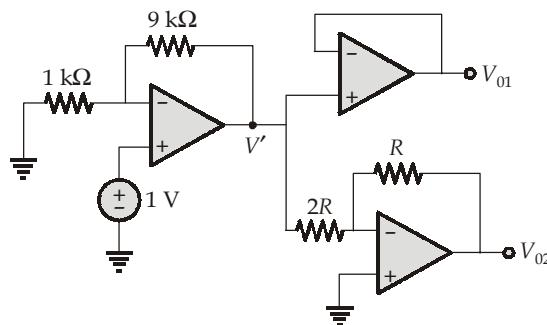
$$V' = \left(1 + \frac{9 \text{ k}\Omega}{1 \text{ k}\Omega}\right) \times 1 \text{ V} \quad (\because \text{non-inverting amplifier})$$
