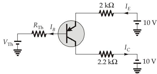
$$\begin{aligned}V_{Th} &= 6.67 \text{ V} \\ R_{Th} &= 10 \text{ k}\Omega \parallel 20 \text{ k}\Omega = 6.67 \text{ k}\Omega\end{aligned}$$
