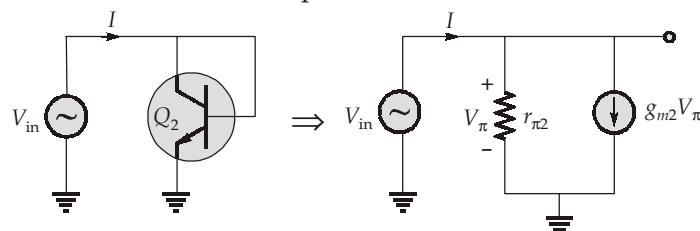
$$\therefore I = \frac{V_\pi}{r_{\pi 2}} + g_{m2} V_\pi$$
