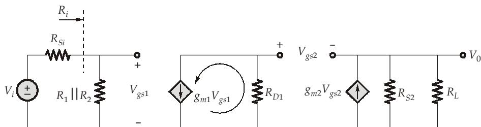
$$\text{Now, } V_0 = g_{m2}(R_{S2} || R_L) \cdot V_{gs2} \quad \dots \text{ (i)}$$
