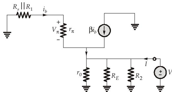
$$\therefore I = \frac{V}{R_2} + \frac{V}{R_E} + \frac{V}{r_0} - (\beta + 1)i_b$$
