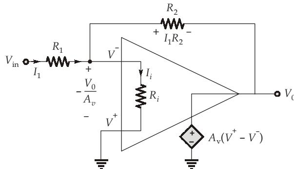
$$V_0 = -\frac{R_2}{R_1} \left[ V_{in} + \frac{V_0}{A_v} \right] - \frac{V_0}{A_v}$$
