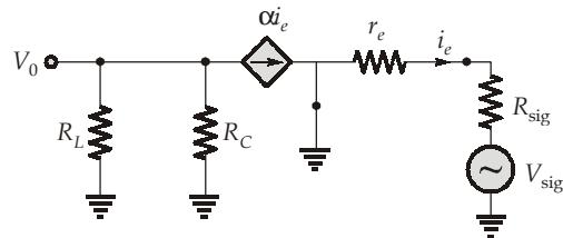
$$V_0 = -\alpha(R_C \parallel R_L) i_e \quad \dots(i)$$
