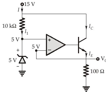
$$I_1 = \frac{15 - 5}{10 \text{ k}\Omega} = 1 \text{ mA}$$
