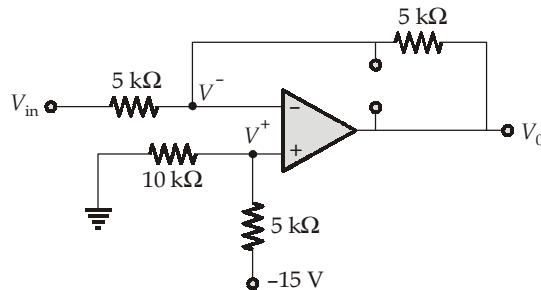
$$\therefore V_0 = -\frac{5}{5} \times V_{in} = -V_{in} \quad (\text{for } V_{in} < -10 \text{ V})$$
