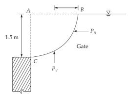
$P_H$  = Force on the projected area of the curved surface on vertical plane
