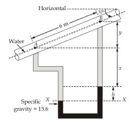
Equating the pressures on both the limbs at the horizontal plane XX ( $y = 6 \sin 37 = 3.6 \text{ m}$ )
