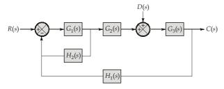
The condition that must be satisfied to remove the effect of disturbance on the response of the system.
