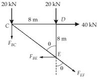
Cut a section through BC, BE and EF and considering its right portion
