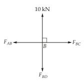
$$\begin{array}{ccc} \therefore & \text{Take} & & \sum F_x &= 0 \\ \Rightarrow & & F_{AB} &= F_{BC} \\ \Rightarrow & & F_{BC} &= \frac{40}{3} \text{kN (T)} \end{array}$$
