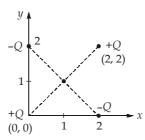
Two positive charges Q are diagonally opposite in position and at the same distance from the point (1, 1, 0) fields produce by them are equal and opposite and so their resultant field is zero. Similarly for negative charges.
