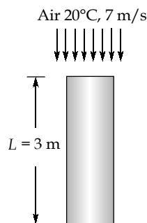
The flow is along 3 m side of the plate, and thus the characteristic length is  $L = 3 \text{ m}$ . Both sides are exposed to air flow,
