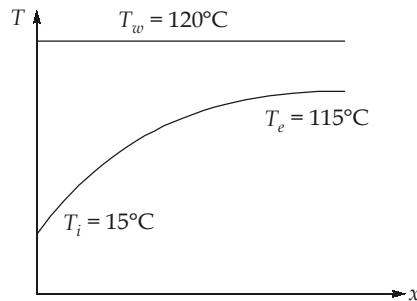
$$\Delta T_i = T_w - T_i = 120 - 15 = 105^\circ\text{C}$$
