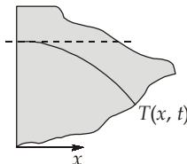
As  $\left.\frac{\partial T}{\partial x}\right|_{x=0} = 0$ , the boundary is an adiabatic or insulated surface.
