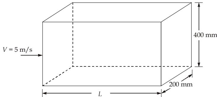
$$\text{Hydraulic diameter, } D_h = \frac{4A}{P} = \frac{4 \times 200 \times 400}{2(200 + 400)}$$
