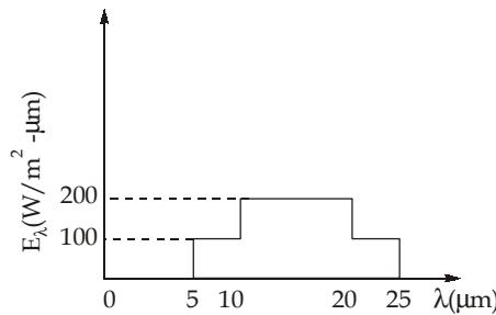
$$E = \int_0^\infty E_\lambda d\lambda = \text{Area under the spectral intensity curve}$$
