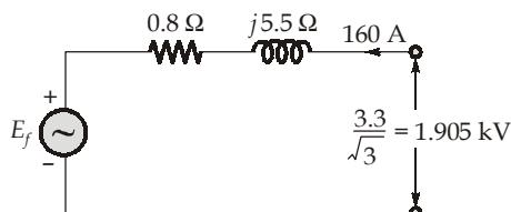
$$\text{Full load current} = 160 \angle -36.86^\circ \text{ A}$$
