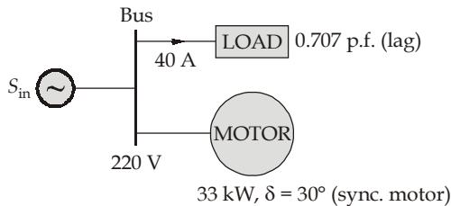
$$\begin{aligned}\vec{S}_{\text{Load}} &= \sqrt{3} \times 220 \times 40 \times \angle \cos^{-1}(0.707) \\ &= 15.242 \angle 45^\circ \text{ kVA} \\ &= (10.78 + j10.78) \text{ kVA}\end{aligned}$$
