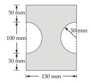
As the section is symmetrical about its horizontal and vertical axis, therefore centre of gravity of section will lie at the centre of rectangle.
