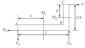
$$= \int_{0}^{l} \frac{M_{x}^{2} dx}{2EI} + \int_{0}^{l/2} \frac{M_{y}^{2} dy}{2EI} = \int_{0}^{l} \frac{\left(-\frac{Px}{2}\right)^{2} dx}{2EI} + \int_{0}^{l/2} \frac{\left(Py\right)^{2} dy}{2EI}$$
