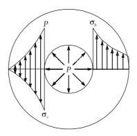
When thick cylinder is subjected to internal pressure 'p', hoop stress (tensile) develops which is maximum at inner radius and minimum at outer radius hyperbolic. The radial stress ( $\sigma_r$ ) develope which is compressive in nature and has maximum magnitude at internal radius and varies hyperbolic to zero value at outer radius.
