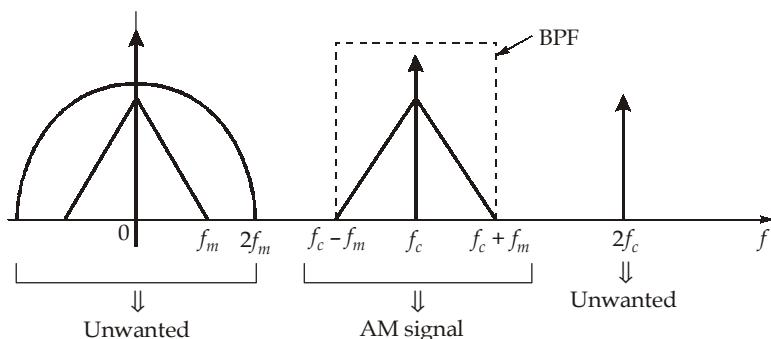
To get the desired AM signal at the output of the filter, the following conditions to be satisfied:
