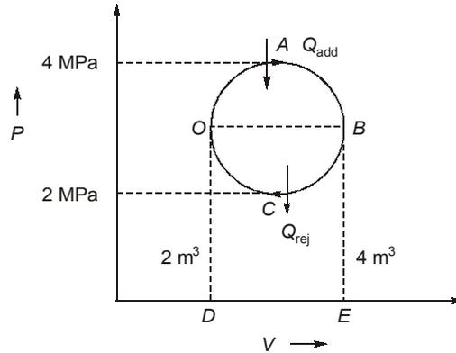
In cycle  $Q_{net} = W_{net} = \text{Area enclosed by cycle.}$
