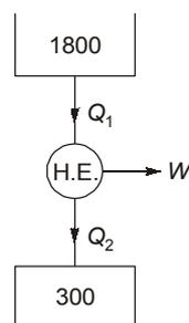
$$\begin{aligned} Q_1 &= 5 \text{ MW} \\ Q_2 &= Q_1 - W = 3 \text{ MW} \end{aligned}$$
