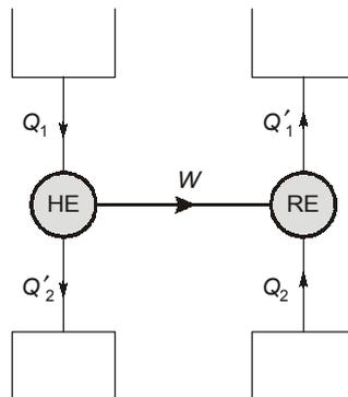
$$\frac{W}{Q_1} = \eta_{\text{engine}} = 0.3 \quad \dots(1)$$
