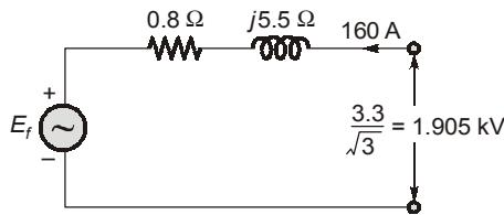
$$\text{Full load current} = 160 \angle -36.86^\circ \text{ A}$$
