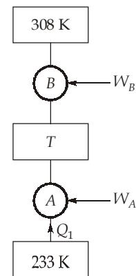
$$W_A = \frac{Q_1}{(\text{COP})_A} = \frac{3}{6.68} \\ = 0.449 \text{ kJ/s} \approx 0.45 \text{ kJ/s}$$
