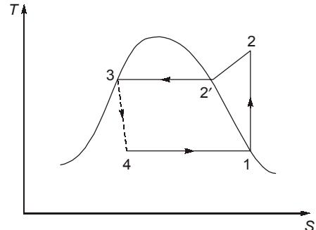
Enthalpy at discharge,  $h_2 = h_{2'} + c_p(T_2 - T_{2'})$
