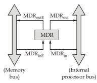
MDR is directly connected to data lines of the processor. It has 2 input and 2 output. Data may be loaded into MDR either from memory or from internal bus. Data present in MDR may be placed on either bus are memory. It requires total 4 control signals.
