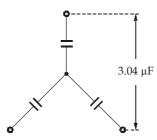
Since the capacitance measured is 3.04  $\mu F$  between the conductors, the capacitance per phase will be
