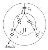
Capacitance between shorted conductors and sheath is  $3C_s$ .
