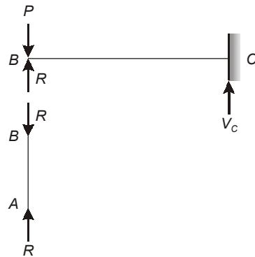
Deflection at A in beam  $BC$  = Compression in column  $AB$
