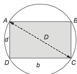
Size of rectangular section ( $b \times d$ ) cutout from circular log of wood
