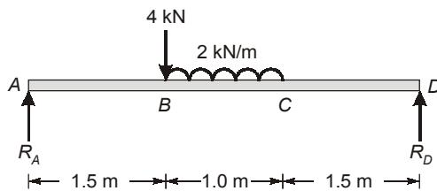
$$\begin{aligned} \Rightarrow \quad & \sum F_y = 0 \\ & R_A + R_D = 4 + 2 \times 1 \\ \Rightarrow \quad & R_A + R_D = 6 \quad \dots(i) \\ \sum M_D = 0 \\ \Rightarrow \quad & R_A \times 4 - 4 \times 2.5 - 2 \times 1 \times 2 = 0 \\ \Rightarrow \quad & R_A = 3.5 \text{ kN} \\ \text{and} \quad & R_D = 6 - 3.5 = 2.5 \text{ kN} \end{aligned}$$
