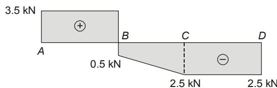
We know that the maximum bending moment will occur at  $B$ , where the shear force changes sign i.e. the distance of point  $B$  from  $A = 1.5 \text{ m}$ .
