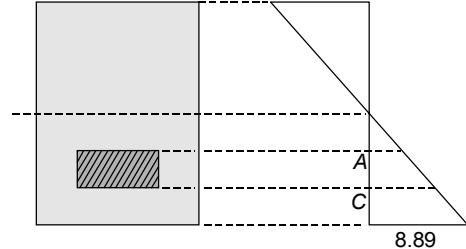
$$\text{Tensile force in hatched area} = \frac{1}{2}(2.96 + 5.93) \times 50 \times 50 = 11.107 \text{ kN}$$
