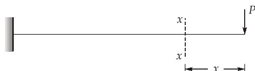
Strain energy stored in a beam due to bending
