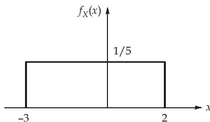
$$\begin{aligned}\therefore N_o &= \int_{-3}^0 \frac{1}{5}(x+1)^2 dx + \int_0^2 \frac{1}{5}(x-2)^2 dx \\ &= \left. \frac{1}{5} \frac{(x+1)^3}{3} \right|_{-3}^0 + \left. \frac{1}{5} \frac{(x-2)^3}{3} \right|_0^2 \\ &= \frac{1}{15}(1+8) + \frac{1}{15}(+8) = \frac{17}{15} \text{ W} = 1.13 \text{ W}\end{aligned}$$
