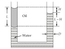
$$L = \frac{V_{oil} \times 4}{\pi D^2} = \frac{3.25 \times 10^3 \times 4}{\pi \times 6.35^2} = 102.623 \text{ mm}$$
