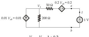
$$0.01 = \frac{V_1}{200} + \frac{V_1 - 1 + 0.2}{50}$$
