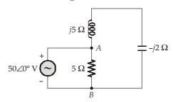
$$V'_{AB} = 50 \angle 0^{\circ} + 0 \text{ V} = 50 \angle 0^{\circ} \text{ V}$$
