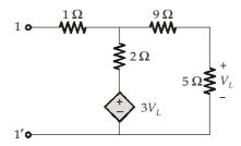
The venin's equivalent resistance of the circuit given from input terminal 1 – 1' will be  $\underline{\hspace{1cm}}$   $\Omega$ .
