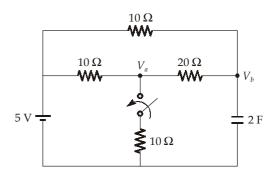
Steady state is reached with switch open. At t = 0, switch is closed then  $V_a(0^+)$  is V.
