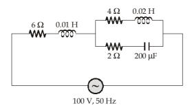
The input power factor is \_\_\_\_\_
