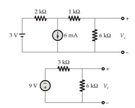
$$v_{c}(\infty) = \frac{6}{9} \times (-9) = -6 \text{ V}$$
