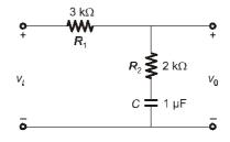
$$G(s) = \frac{V_0(s)}{V_i(s)} = \frac{R_2 + \frac{1}{sC}}{R_1 + R_2 + \frac{1}{sC}}$$
