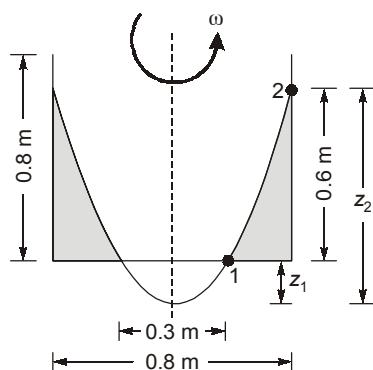
$$z_2 - z_1 = \frac{\omega^2}{2g} [R_2^2 - R_1^2]$$
