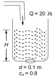
Assume  $H$  is the level of water in the tank in steady condition.
