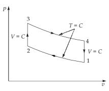
The cycle takes in air at 1 bar and 300 K. The air is compressed isothermally and then heated at constant volume so that the pressure rises to 15 bar and temperature to 700 K. The air expands isothermally to its initial volume and rejects the cycle. What is the mean effective pressure?
