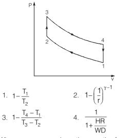
Where, r = compression ratio, g = ratio of specific heats, HR = heat rejected, WD = work done Which of the above expressions are correct?
