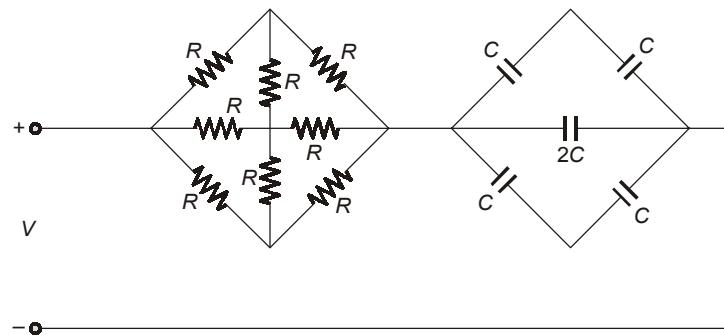
The time constant of an  $RC$  circuit is  $\tau = R_{\text{eq}} C_{\text{eq}}$
