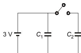
$C_1$  gets charged upto 3 V charge stored in  $C_1$
