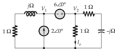
$$\frac{V_1}{1+j} - 2 + \frac{V_2}{1} + \frac{V_2}{1-j} = 0$$
