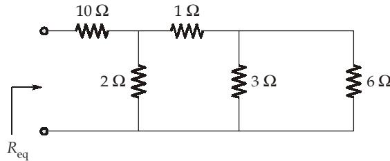
$$\therefore R_{\text{eq}} = 10 \Omega + 2 \Omega \parallel (1 + 3 \Omega \parallel 6 \Omega)$$
