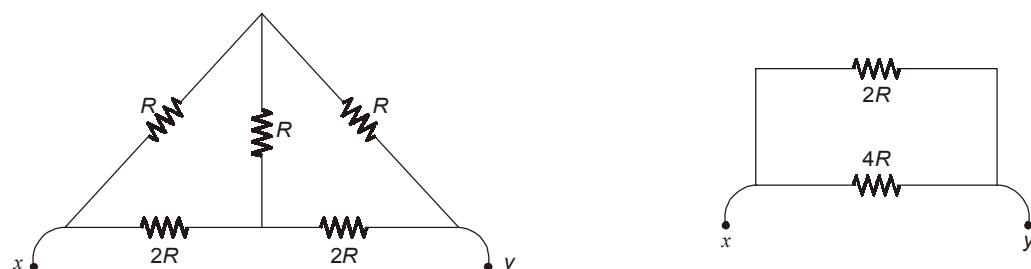
$$(R_{\text{eq}})_{\text{Half circuit}} = \frac{4R \times 2R}{6R} = \frac{4R}{3}$$
