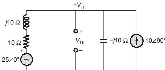
$$\frac{V_{Th} - 25}{10 + j10} + \frac{V_{Th}}{-j10} = 10\angle 90^\circ$$
